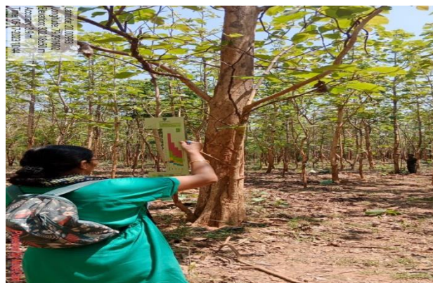
Figure 4. Height measurement with Hypsometer
