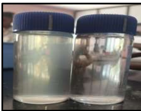
Fig.4. Turbidity- before and after treatment with bioadsorbent
