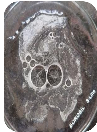
Bioenzyme solution Drop collapse
