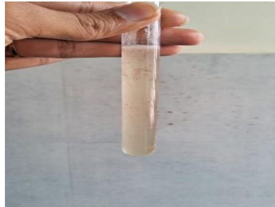
Oil-Water Emulsion treated with Bio enzyme solution
