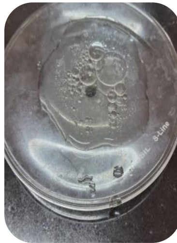
1% SDS solution Drop collapse Drop collapse Method
