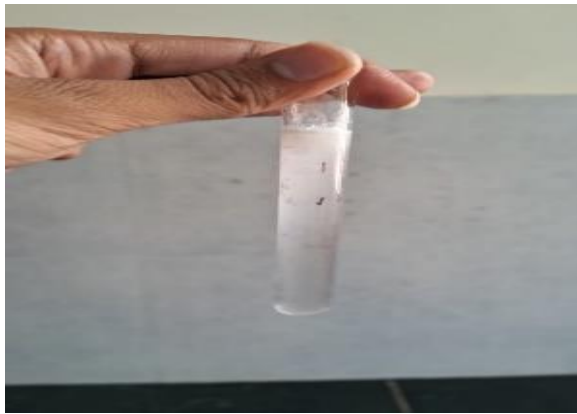
Oil-Water emulsion treated with 1% SDS solution
