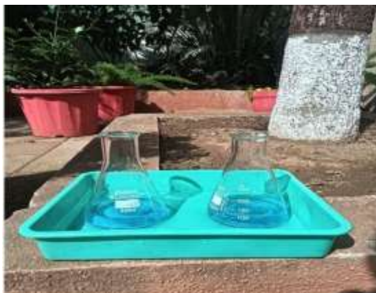
Figure 5: Experimental setup for photocatalytic degradation of MB under sunlight
