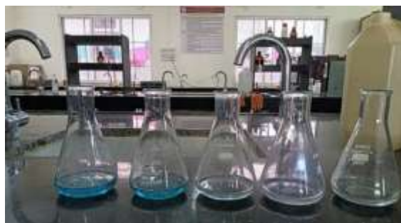
Figure 10: M B degradation with irradiation time using ZnO photocatalyst.
